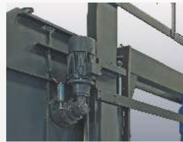
High efficiency power transmission to Saw through PLANETARY GEAR BOX
