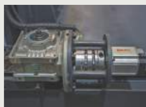
Indexing of Heads thru Servo Motor coupled with the Gear Box.
