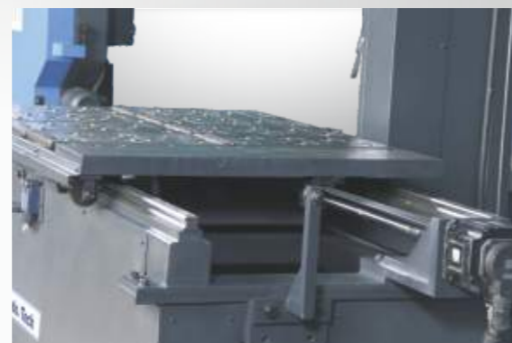
Main Table Indexing through Servo Drive System for precise cuts
