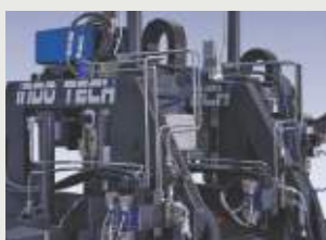
Dual Cutting Heads for independent Drilling & Tapping spindles.
