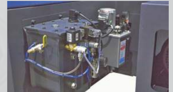
Mist Cooling System
