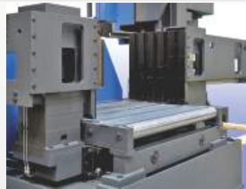
Hydraulic Auto indexing shuttle with much wider & heavy vices to pull heavy loads and synchronized with auto cycle
