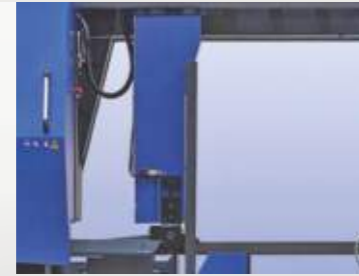
Automatically Adjustable, Dove-tail Type Heavy Duty Movable Blade Guide with hydraulic locking facility.
