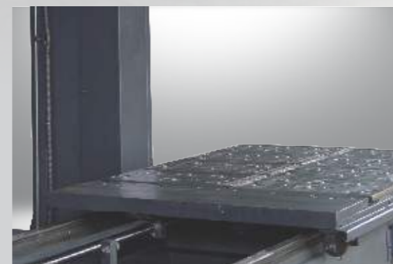
Multiple Ball Transfer Units on Main Table for easy handling of Heavier Jobs
