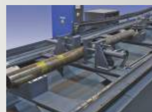
Multiple Fixed Hydraulic Clamping vices with V-block resting.
