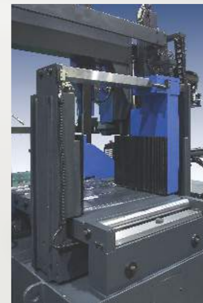
Specially designed heavy duty Bridge type Job Clamping & Indexing Shuttle
